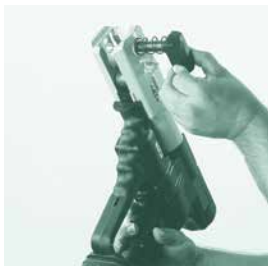
Open the retaining pin at the front of the machine by pressing the jaw to release button*.
