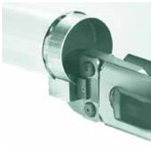
Release the jaw then press the trigger and lug the pipe until a "snap" is heard.
