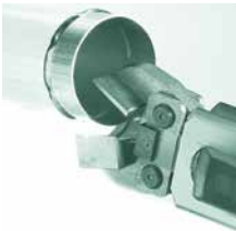
Manually open the jaw and insert the stainless steel pipe until the pipe meets the stop in the jaw.
