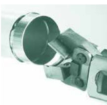
Re-open the jaw to remove the pipe. Position the end of the jaw next to the lug mark: this will help to prevent overlapping the lugs.
