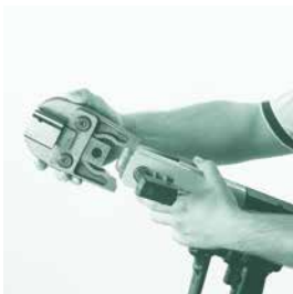
Place the jaw in the housing.
