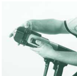
Lock into position by closing the retaining pin.
