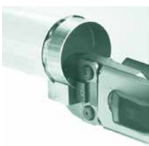
Repeat the operation until the required minimum of lugs for each diameter have been achieved.
